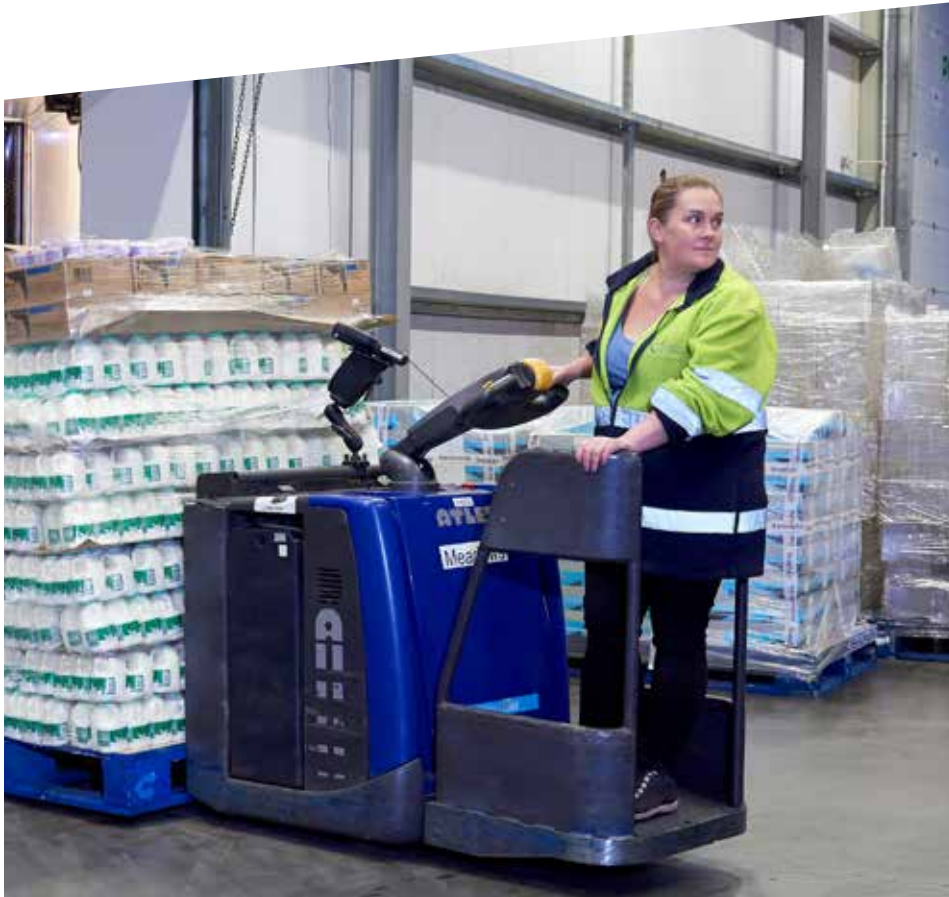
PMR pallet trucks used to load and unload trucks and transfer pallets
