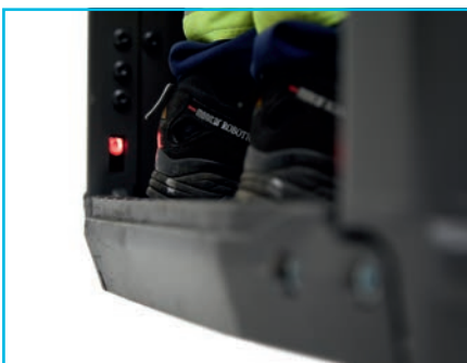
Foot protection option stops the truck automatically when the driver's feet move off the platform.
