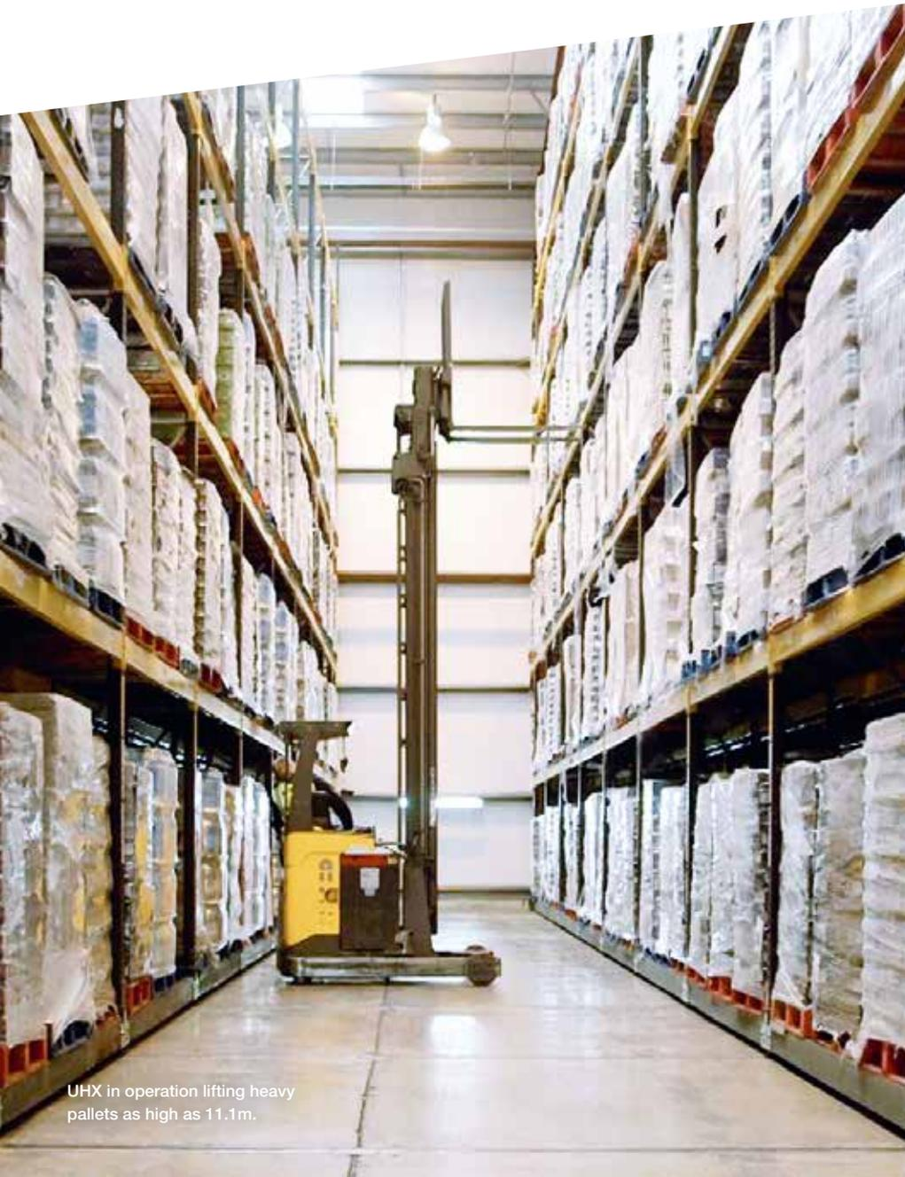
UHX in operation lifting heavy pallets as high as 11.1m.
